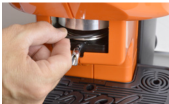
Insertion of a new gasket
