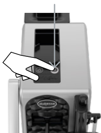
Fig. 9-D - press the milk dispensing button: the LED will flash during heating and will remain steady once the temperature is reached
