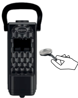
Fig. 12-B - pull out the pod holder
