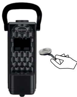
Fig. 12-B - pull out the pod holder
